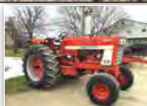
IHC 1066, 2WD, Factory open station, 2 remotes, 540/1000 PTO, 20.8 x 38 tires, exc con, Stk# 0862995
