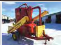
NH 358 MIXMILL hyd, scale, 540 PTO, 20' unload, good con, Stk# 0863000
