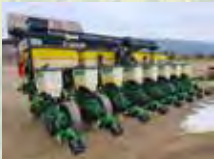
JD 1750 8 row, XP row units, vDrive, DeltaForce, Hyd drive dry fert, Gen 3 20/20
