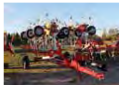
POTTINGER HIT 12.14T tedder, 43' working width
