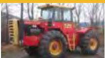
Versatile 500 Tractor 1978, 4WD, 1000 PTO, 3 Sets Rear Remotes, 23.1 - 30 Tires, Runs and Drives Well 200 HP 5500 HRS $18,900
